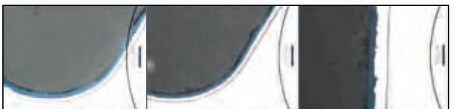
Micrographs of coatings on studbolts
